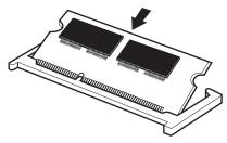
(Sample Illustration) Inserting the module in the socket
